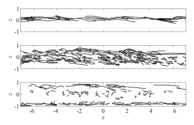
FIG. 3. Sample binary edge frames ( $\mathcal{E}$  space), delineating the locations of sharp density interfaces (black), mapped from the shadowgraphs ( $\mathcal{E}$  space) of Fig. 1(c) in the three human-classified regimes: Holmboe (H, top), intermittent (I, middle), and turbulent (T, bottom). Edges are here rendered much thicker than detected for better visualization.
