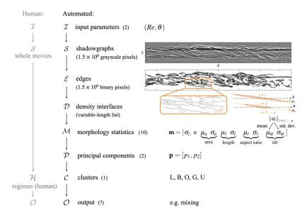
FIG. 2. Dimensionality reduction pipeline used to assign a cluster label to each shadowgraph frame. The spaces and successive mappings of the new automated classification approach (second column from left, in black) are compared to the traditional human approach (left, in gray). The bracketed numbers indicate the dimension of each space, highlighting a dramatic reduction in dimensionality.
