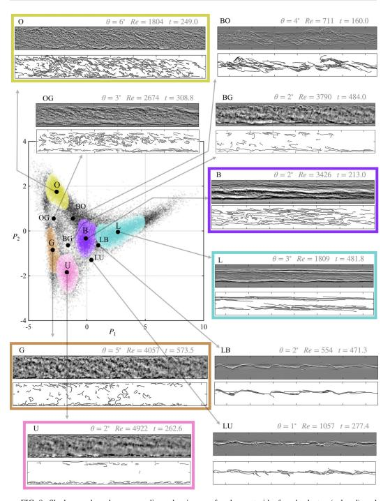
FIG. 8. Shadowgraph and corresponding edge images for the centroid of each cluster (colored) and additional examples of frames between clusters. The input parameters (Re,  $\theta$ ) and time t are indicated in the top-right corner of each frame. Frames are scaled to have equal height, resulting in a range of lengths.
