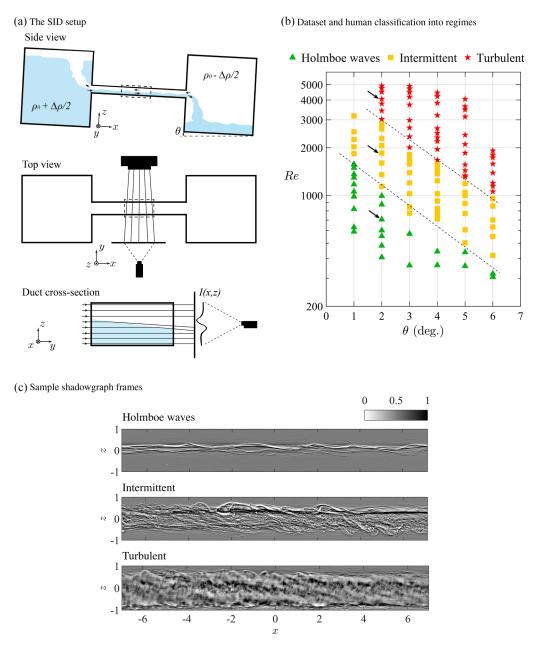
FIG. 1. Experimental data. (a) Sketch of the setup and shadowgraph measurements used to visualize the density field. (b) The 113 experiments in the space of input parameters (Re,  $\theta$ ) labeled with their human classified regime. The dashed lines roughly highlight regime transitions. Three arrows indicate the locations of the sample shadowgraph frames  $\tilde{I}(x, z)$  presented in (c). The original images are  $\approx 3400 \times 450$  pixels.
